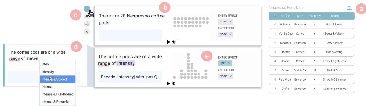
Figure 5: A user setting up and adding blocks to develop a story with DataParticles. When the user (a) imports data to set up the story, DataParticles (b) automatically generates the first block enabling the user to (c) add a block and (d) write a story using natural language. The system (e) shows the corresponding visualization while the user is writing.
